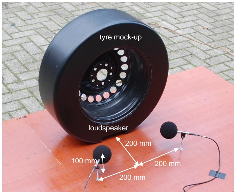
figure 4 The measurement setup used to determine the device correction
